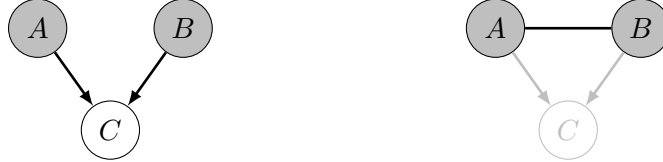
Figure 4.5: Moralization of a graph. Left: Joint distribution. Right: Conditional distribution of the parents given the offspring.
